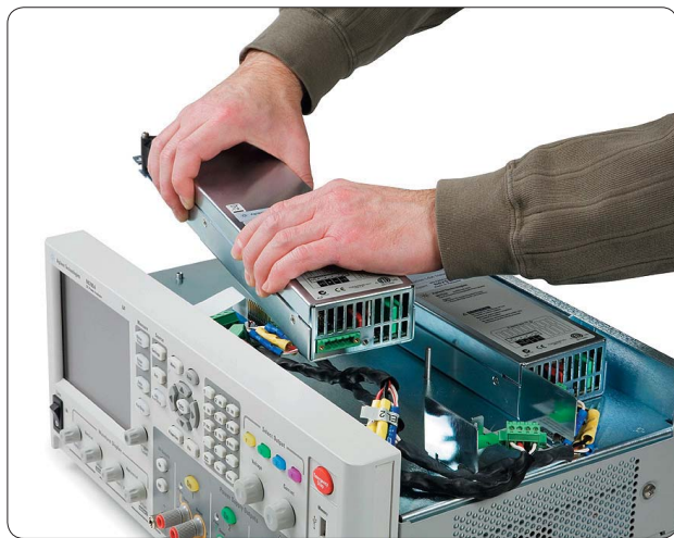
Figure 2. DC power modules are easily installed into the N6705 DC power analyzer mainframe.
